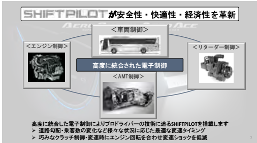
バスのAMT統合制御 AMT Integrated Control for buses (Shift Pilot)
